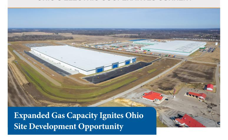
Over 20 years ago, Consolidated Cooperative, the local electric, fiber and gas cooperative, purchased some unused gas well gathering lines in Morrow County, Ohio. The cooperative engineered the reversal of the pressure to turn the lines into a distribution system that provides natural gas service to commercial development around the I-71/SR 61 interchange in central Ohio.
